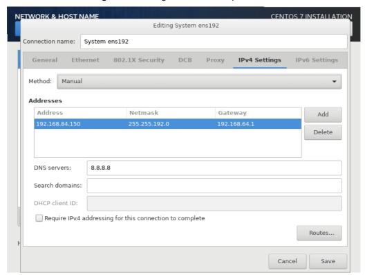
"Method" should be configured as "Manual", this will allow you to configure a static IP address to the Backup Server/Backup Node. Then click on "Add" to manually configure the network profiles. And in the "DNS servers" field, insert a valid DNS server IP. When done, click on "Save".
