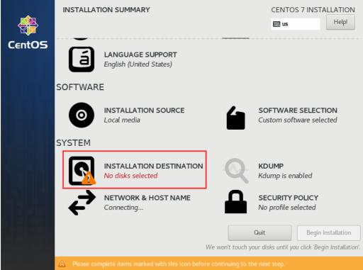
Select the target disk, and you can choose "Automatically configure partitioning" to let the system automatically do the partitioning. Or if you have other plans with the disk, you can choose "I will configure partitioning" to manually configure the disk partitioning.
