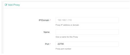
Simply input the IP address of the Backup Proxy in the "IP/Domain" field.
